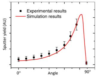
The milling efficiency is a function of the local curvature of the sample. Milling works most efficiently between 75-85°. At 90° the sputter yield is near zero. Hence, do not mill samples that are not flat: you will end up with a preferentially milled object.
