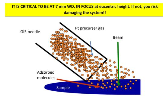
Note: Pt deposition is usually done with the ion beam, but can also be perforned with the electron beam
