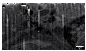
materials with different sputtering yields, the ion beam removes material at different rates, leading to uneven surfaces. The polishing step reduces the curtaining effect.
