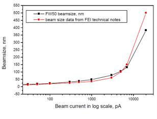
The higher the ion current, the wider, larger the ion beam.
