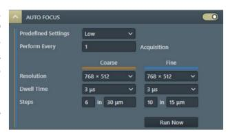
the working distance in a two-step approach over a specified range while measuring image sharpness. First a Coarse sweep (orange color) to get close to focus is perfromed, followed by a Fine sweep (blue color) to optimize it. Tune the parameters – the autofocus needs a good quality image - and run the auto focus prior to starting a project execution.
