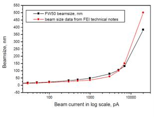
The higher the ion current, the wider, larger the ion beam.
