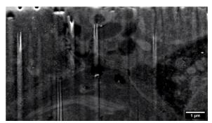
materials with different sputtering yields, the ion beam removes material at different rates, leading to uneven surfaces. The polishing step reduces the curtaining effect.
