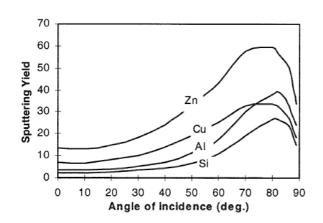
Similar to the Mohs scale of hardness of solids (graphene = soft, diamond is hard), each material has a tendency to get sputtered by the Ga ion beam. The sputter rates are not a function of the Mohs scale.
