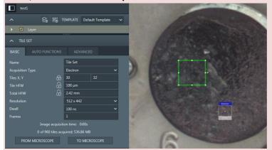
This reads the settings of the microscope and calculates the number of tiles that are required. The image is updated:
