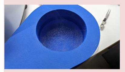
Lift the lid of the cryotransfer container and place it in the liquid nitrogen container. Assure the lid of the cryo box is open (place the transfer tool with the lid or the handling rod submerged in the blue styrofoam shuttle. Cover with the Styrofoam lid as much as possible.
