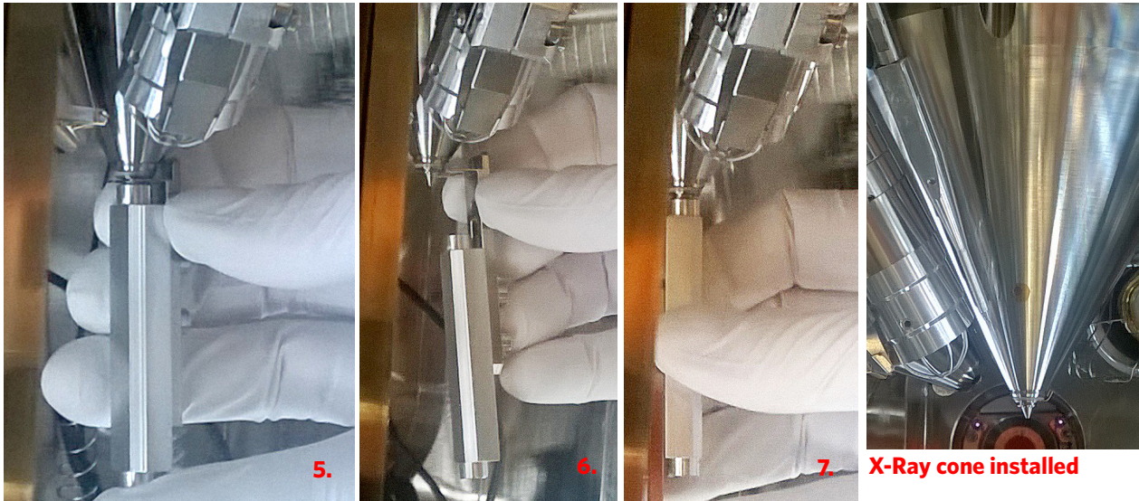
FIGURE 5-5 X-Ray Cone mounting Procedure
