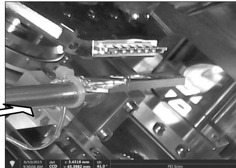
No TEM grid manipulation; the samples are made and imaged without manipulating sample or breaking the vacuum
