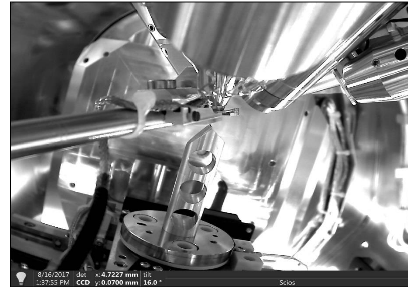
choosing single stub holder; sw restrictions are disabled
