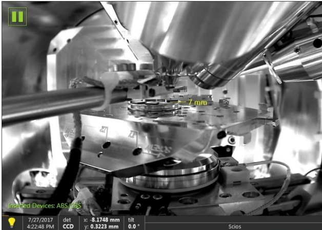
tilt restrictions using large holder
